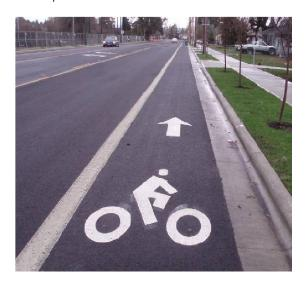
Typically located on curb and gutter roads, and most appropriate for arterial and collector roads, main sections of the network connections expected to experience higher cyclist and/or motor vehicle volumes.
